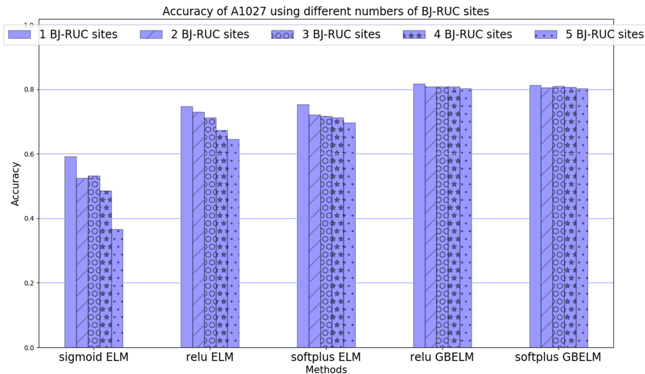
Fig. 5. The accuracy of five methods using different numbers of nearest BJ-RUC forecasting sites in A1027 road monitor station.
